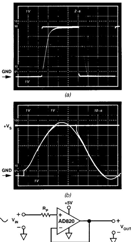
図36(a).  $R_p = 0$  での応答 ( $V_{IN} = 0 \sim +V_S$ )
