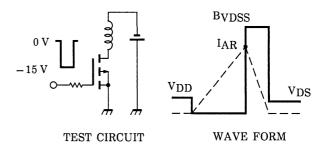
$$\begin{array}{ll} T_{ch} = 25^{\circ} C \; (Initial) \\ Peak \; I_{AR} = -7 \; A, \; R_G = 25 \; \Omega \end{array} \quad E_{AS} = \frac{1}{2} \cdot L \cdot I^2 \cdot (\frac{B_{VDSS}}{B_{VDSS} - V_{DD}}) \\ V_{DD} = -24 \; V, \; L = 1.0 \; mH \end{array}$$
