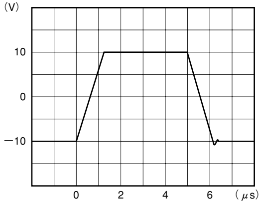
パルス応答特性 1 ( V^\pm = \pm 15\text{ V} , A_v = +1 ) ( R_L = 2\text{ k}\Omega , C_L = 100\text{ pF} )
