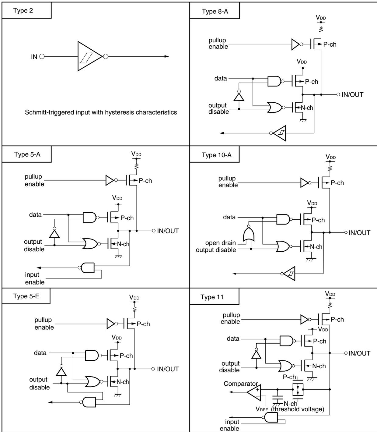
Figure 2-1. List of Pin Input/Output Circuits (2/2)
