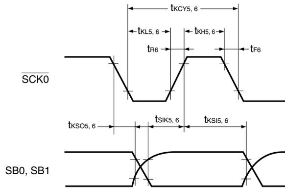
3-wire serial I/O mode with automatic transmit/receive function:
